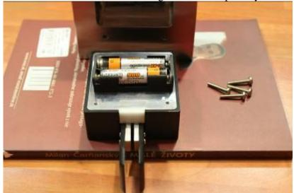
8. Put batteries in holder, while taking care that the polarity is correct.
